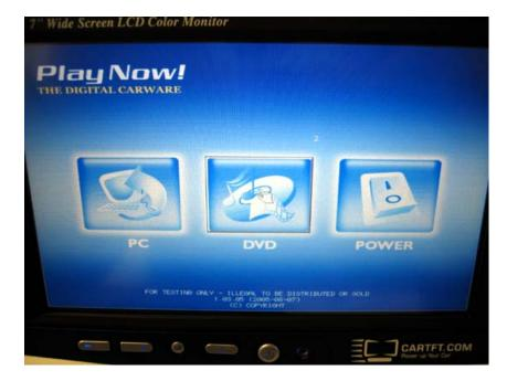
At the case front buttons or keyboard you can select, whether the O/S shall be started now **(PC)** or a DVD shall be played without loading the O/S before **(DVD)** or whether you want to turn the PC off **(I/O)**.
