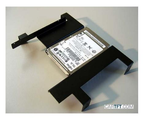
Then drive through the IDE cable under the inner framework and attach it to the HDD.
