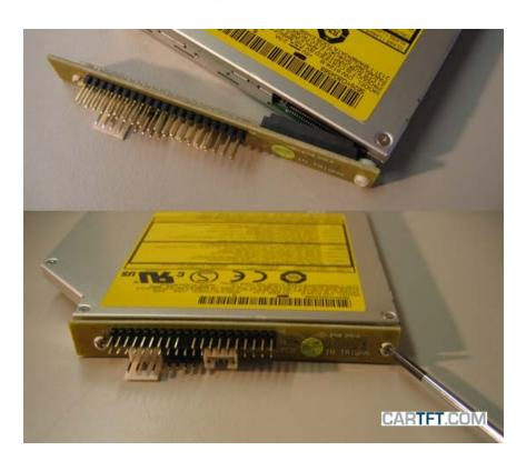
Sliding now the Slimline disk drive of the front into the track by the case disk drive slit until the screw holes of the Slimline disk drive lie at the 2 corresponding openings  $\rightarrow$  then screw them tight.
