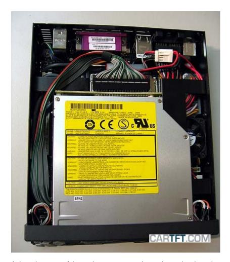
At last, the cover of the casing gets screwed onto the casing, but take care that no cable gets jammed in or gets damaged. Now the InDash V2 Car PC has been assembled completely.
