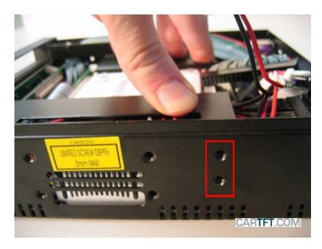
The power connection gets connected to the HDD..
